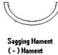
BM is said to positive if moment on left side of beam is clockwise or right side of the beam is counter clockwise.
