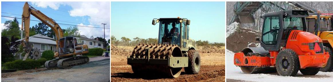
In geotechnical engineering, soil compaction is the process in which a stress applied to a soil causes densification as air is displaced from the pores between the soil grains. When stress is applied that causes densification due to water (or other liquid) being displaced from between the soil grains, then consolidation, not compaction, has occurred. Normally, compaction is the result of heavy machinery compressing the soil, but it can also occur due to the passage of (e.g.) animal feet.
