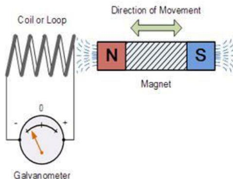
Consider a magnet approaching towards a coil. Here we consider two instants at time  $T_1$  and time  $T_2$ .
