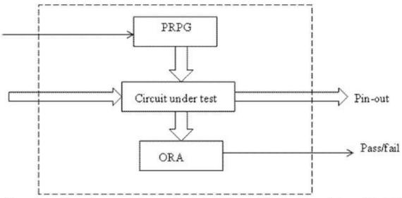
The roles of there two modules are illustrated above. The implementation of both PRPG and DRA can be done with linear feedback shift registers (LFs Rs)
