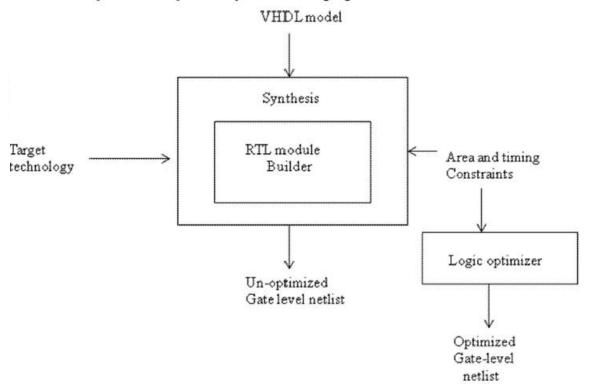
A synthesis process may alternately a RTL net list, which is comprised of generate Register - Transfer level blocks.
