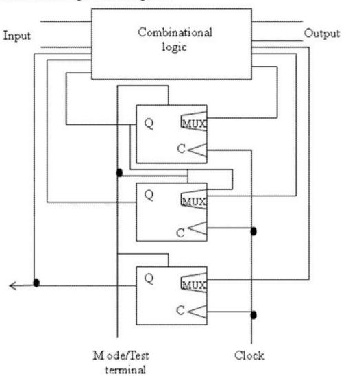
Step 7: Return to test made, scan-out the contents of the registers, and at the same time scan-in next pattern.
