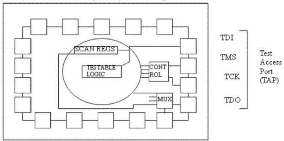
The boundary scan path is provided serial input and output pads and appropriate clock pole which make it possible to
