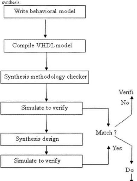
In this design process, a synthesis methodology checker is needed to check if the model being written is compatible for synthesis or not. This is done in the first Simulation loop. In this way, after the Simulation results have been verified, a verified synthesizable model exists, which can then be synthesized.
