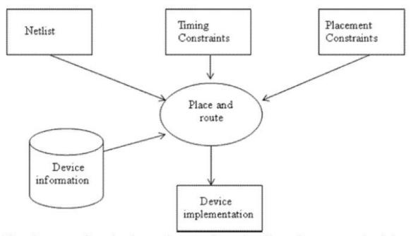
The other output from the place and route software is a file used to generate the timing file. This file describes the actual timing of the programmed FPGA deice or the final ASIC deice.
