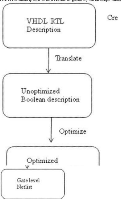
The RTL description at first is converted to a un optimized Boolean description which consists of basic gates, flip flops and latches. This is functionally correct but completely an unoptimized description. Next, Boolean optimization algorithms are executed on this Boolean equivalent description to produce a optimized Boolean equivalent description. Finally this is mapped to acheal logic gates by using technology library of target process. Each stage is explained below:
