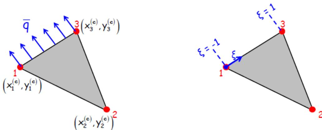
In this case, segment (1-3) is a boundary segment, so we can introduce the parameterization shown above. Now, we can express the values of x and y along the natural boundary segment as functions of  $\xi$ :
