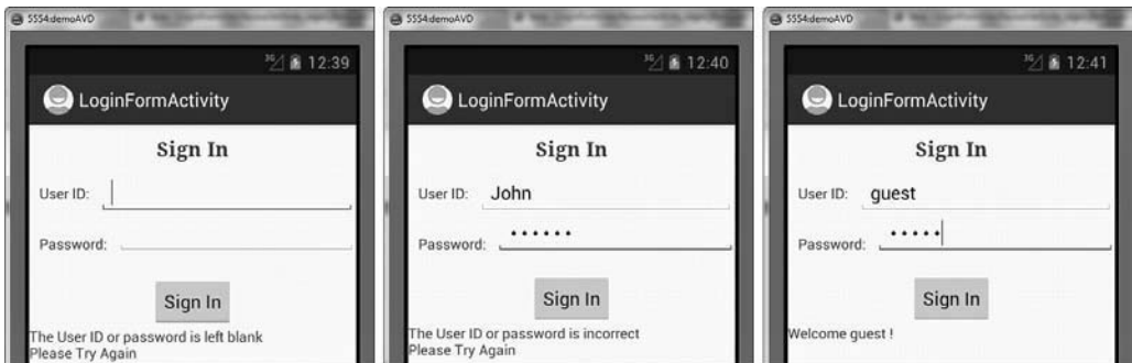
FIGURE 3.10 (left) The Login Form displays an error if fields are left blank, (middle) the Password Incorrect message displays if the user ID or password is incorrect, and (right) the Welcome message displays when the correct user ID and password are entered.
