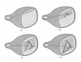
The electron beam is swept across the screen one row at a time from top to bottom. As it moves across each row, the beam intensity is turned on and off to create a pattern of illuminated spots. This scanning process is called refreshing. Each complete scanning of a screen is normally called a **frame**.
