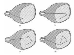
The CRT's electron beam is directed only to the parts of the screen where a picture is to be drawn. The picture definition is stored as a set of line-drawing commands in a refresh display file or a refresh buffer in memory.
