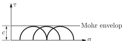
Slope of mohr envelope is zero,  $\phi$  is zero.
