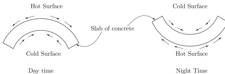
But due to self weight opposite stresses are introduced i.e. compressive on top and tensile at bottom during day time, tensile on top and compressive at bottom during Night time.
