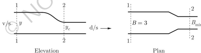
We have find width of section 2-2 ' $B_{min}$ ' at which the depth reaches critical depth ' $y_c$ ' and specific energy is  $E_c$
