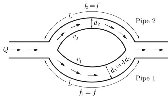
Let the velocity in upper pipe be  $V_2$  & in lower pipe be  $V_1$ ,  $Q$  is the original discharge.
