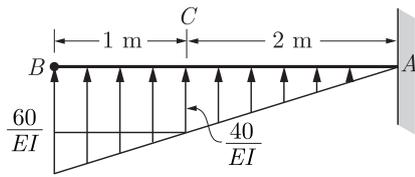
Deflection at C due to this loading is Bending moment of conjugate beam diagram at C, which is 2 mm (given)
