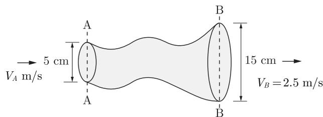
Given velocity at  $B-B$  section is  $2.5$  m/s & velocity at section  $A-B$  is  $V_A$  m/s.
