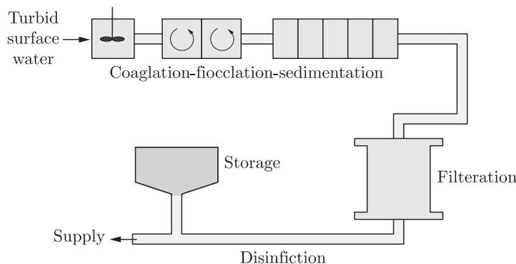
Turbid water is coagulated by adding agents like Alum etc to water after which they form flocks of colloids which are heavy enough to sink. Therefore sedimentation is carried out after that. Further, the water is filtrated and made free of microorganism by disinfection process.
