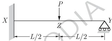
For collapse mechanism to form, a plastic hinge should form at  $X$  and then below the load at  $Z$ . There is a real hinge at  $Y$ .
