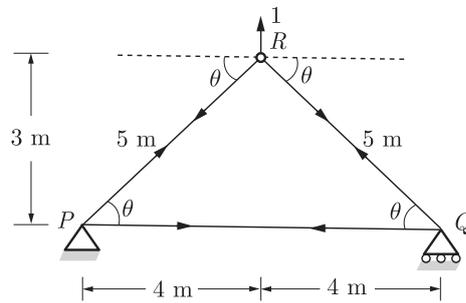
by method of joints at  $R$ ;  $\Sigma F_x = 0$
