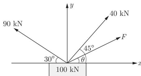
Making free body diagram of box and breaking forces into components in  $x$  &  $y$  direction.
