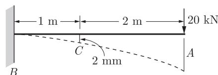
If flexural rigidity of beam be  $EI$  so conjugate beam diagram of beam  $AB$  (i.e.  $M/EI$  diagram)
