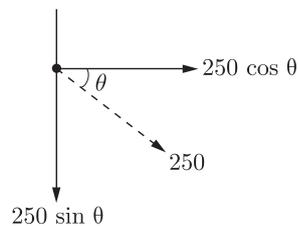
So Tension on joint is  $250 \cos \theta = 250 \times \frac{4}{5} = 200 \text{ kN}$
