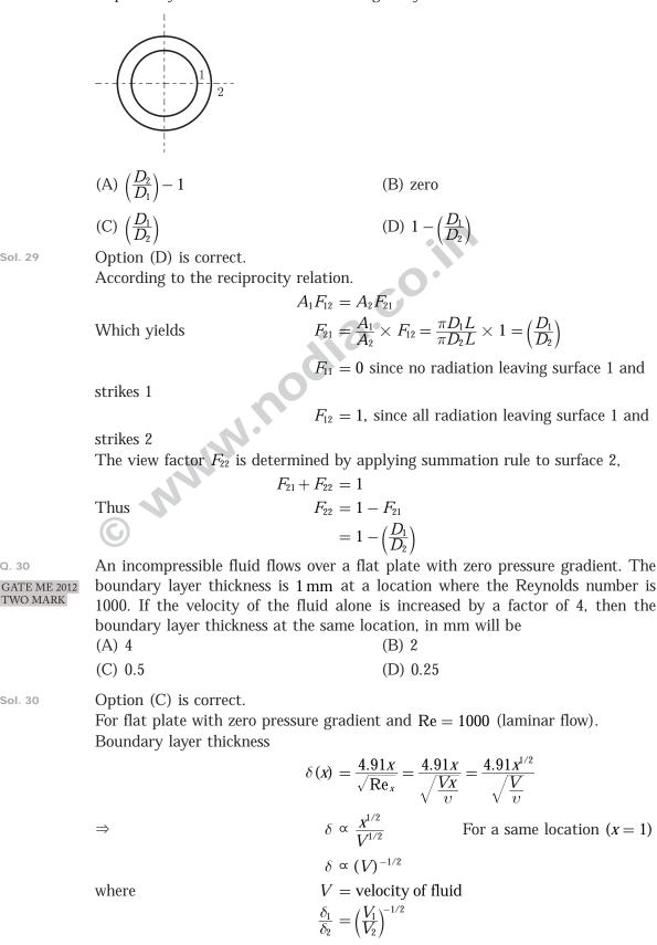
$$\begin{split} \delta_2 &= \left(\frac{V_1}{V_2}\right)^{1/2} \times \delta_1 = \left(\frac{V_1}{4V_1}\right)^{1/2} \times 1 \ V_2 = 4 \ V_1 \ \text{(Given)} \\ \delta_2 &= \left(\frac{1}{4}\right)^{1/2} \times 1 = \frac{1}{2} = 0.5 \end{split}$$
