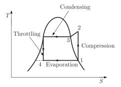
T-s diagram for given Refrigeration cycle is given above Since Heat is extracted in evaporation process. So rate of heat extracted
