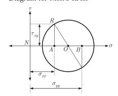
Given,  $\sigma_{xx} = 40 \text{ MPa} = AN$ ,  $\sigma_{yy} = 100 \text{ MPa} = BN$ ,  $\tau_{xy} = 40 \text{ MPa} = AR$ Radius of Mohr's circle
