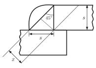
The shear strength of the joint for single parallel fillet weld is,
