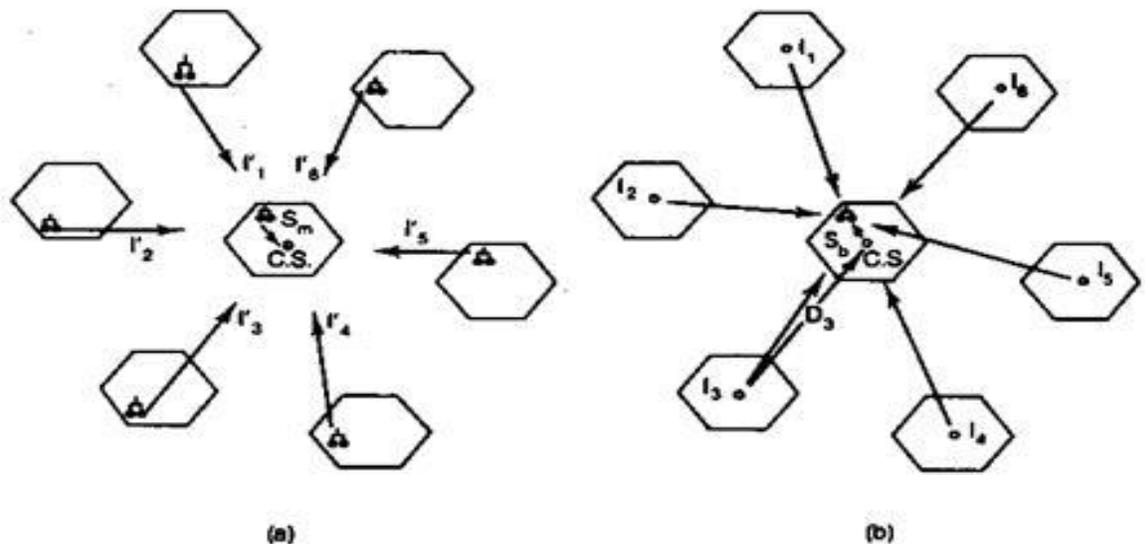
**Fig 2.4 Cochannel interference from six interferers. (a).receiving at the cell site; (b) receiving at the mobile unit.**
