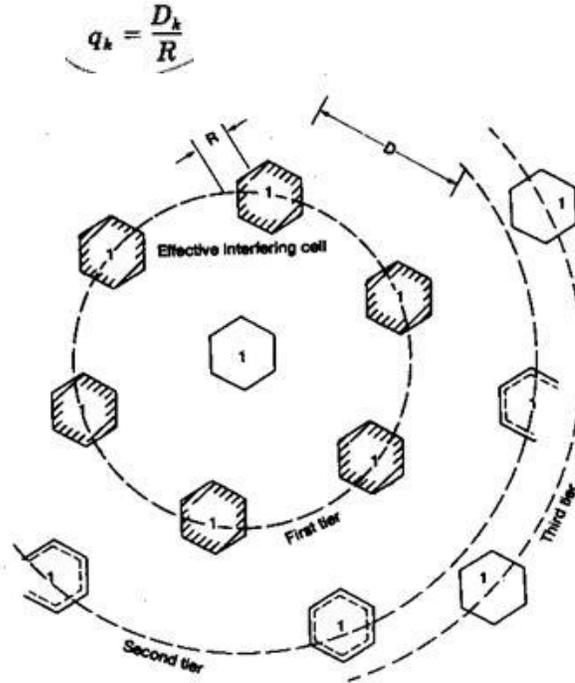
Fig 2.3: Six effective interfering cells of cell 1
