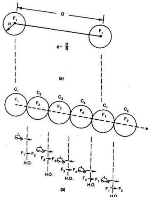
**Fig.2.5: (a). cochannel interference reduction ratio 2, (b) fill in frequency need of splitting**
